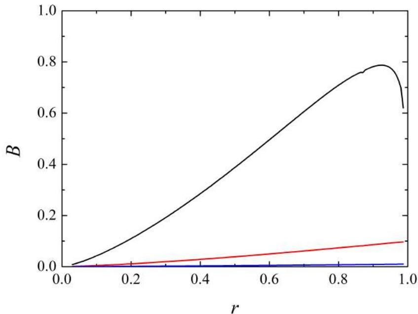
Figure 3. Structure of the magnetic field induced by outflows. Black line shows  $\beta = 1$ , red line –  $\beta = 10$ , blue line –  $\beta = 100$ .
