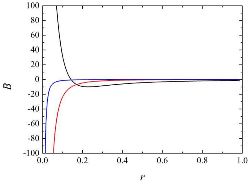
Figure 2. Structure of the magnetic field induced by the radial flows. Black line shows  $\chi = 1$ , red line –  $\chi = 10$ , blue line –  $\chi = 100$ .
