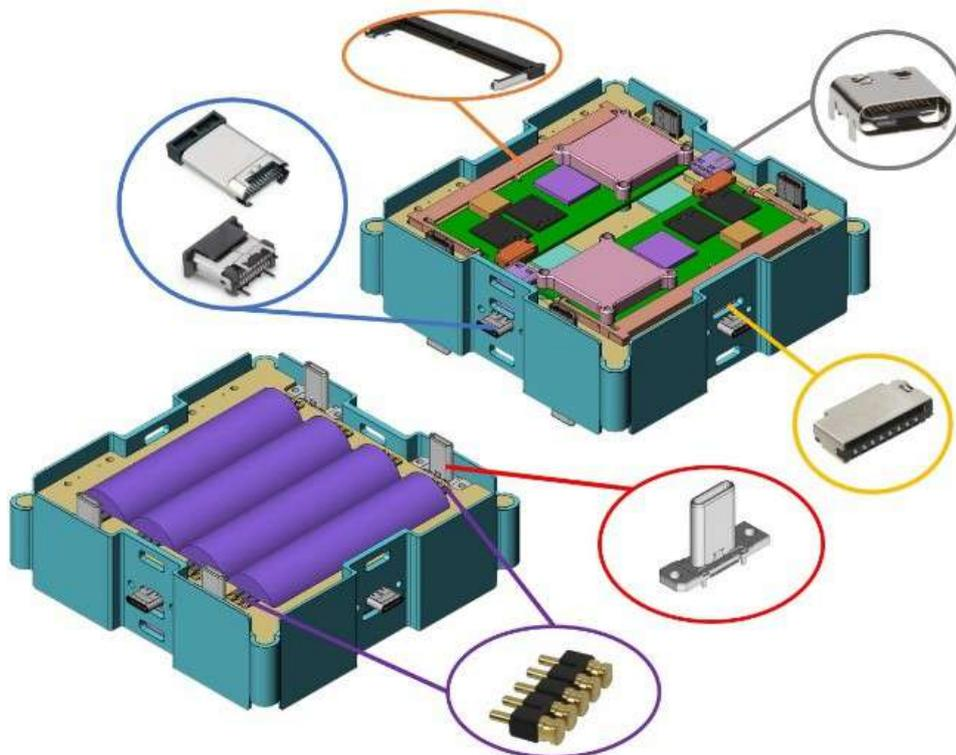
Figure 2. Internal configuration of the nanosatellite.
