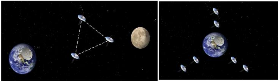
Figure 2. Variants of the ground-to-space antenna array using precise small antennas in space arm of the interferometer.
