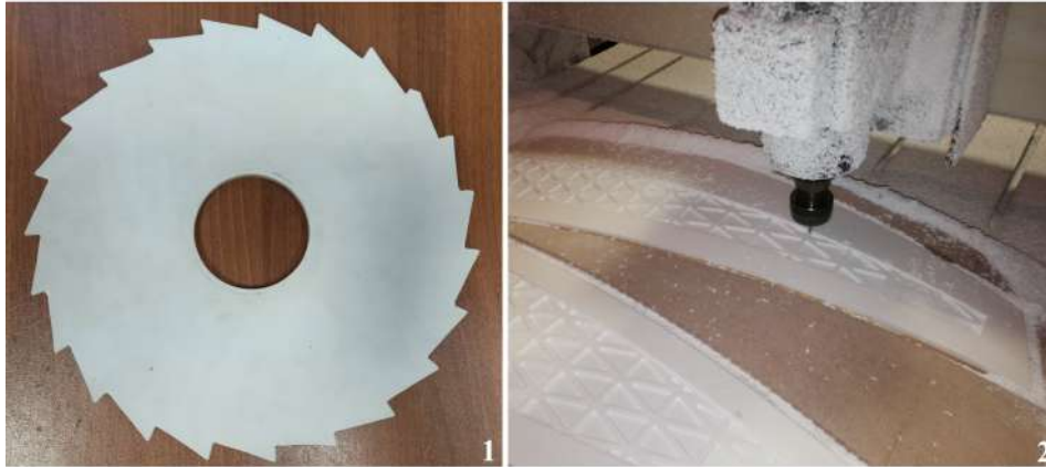
Figure 9. 1 - Central mirror of the composite parabolic reflector, 2 - Manufacturing of stiffeners of the parabolic element of the composite mirror on CNC.
