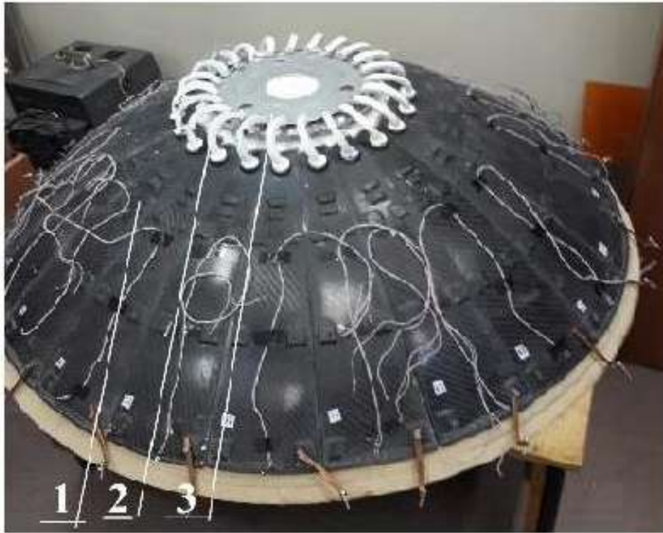
Figure 13. Assembly of a petal mirror on a parabolic template. 1 - petals, 2 - curvilinear rod connecting the petal with the base of the central mirror 3 - the base of the central mirror.
