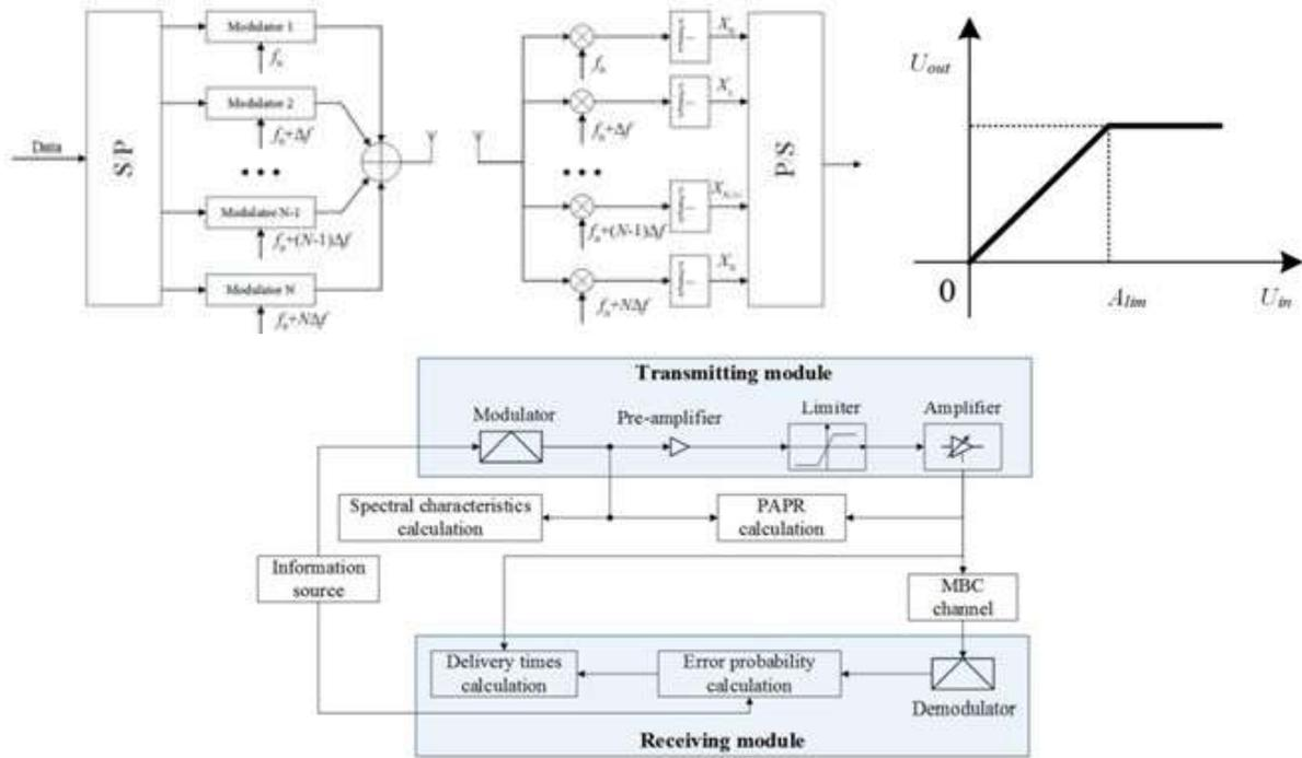
Figure 2. Formation and reception of OFDM signals (on the left), Characteristic of the limiter (on the right), Simulation model (on the bottom).
