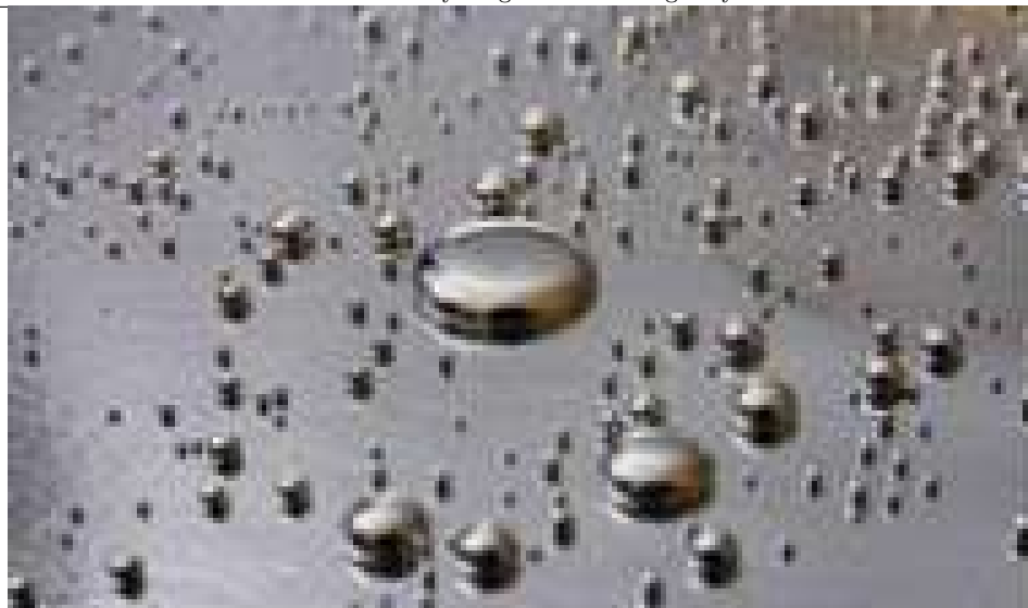
Figure 5. Spherical fragments of various masses formed when the vessel filled with mercury is destroyed.
