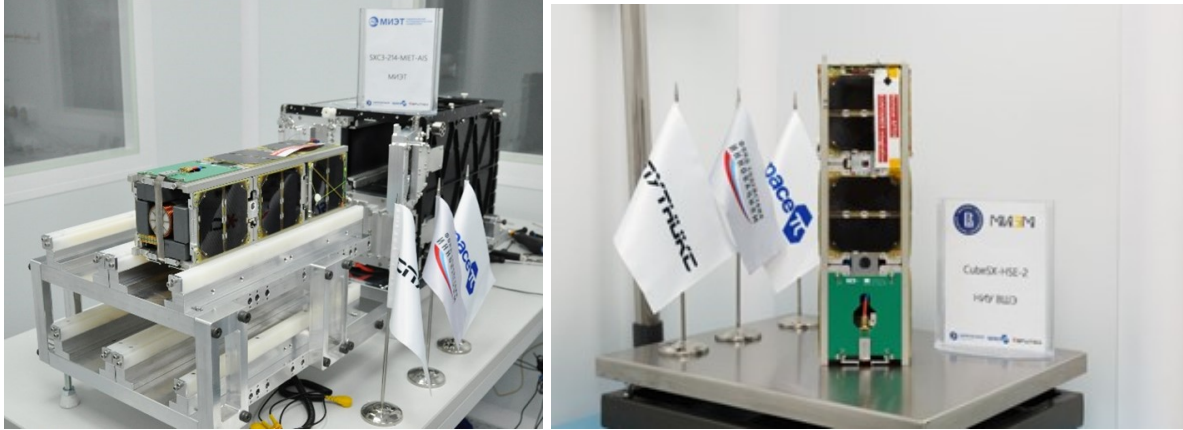
Figure 1. Left: spacecraft CubeSat 3U SXC3-214-MIET-AIS, on which the onboard receiver of AIS signals is installed. Right: spacecraft CubeSX-HSE-2, on which the onboard receiver of AIS signals is installed.)
