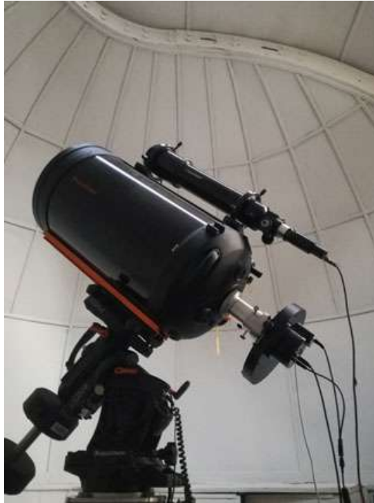
Figure 5. The SCT-14 equipped with the Starlight Express SX-36 CCD, UBVRI filter set and guiding system.
