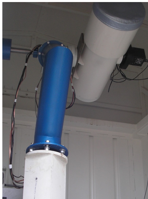
Figure 5. 250 mm aperture telescope mounted in the container-dome.
