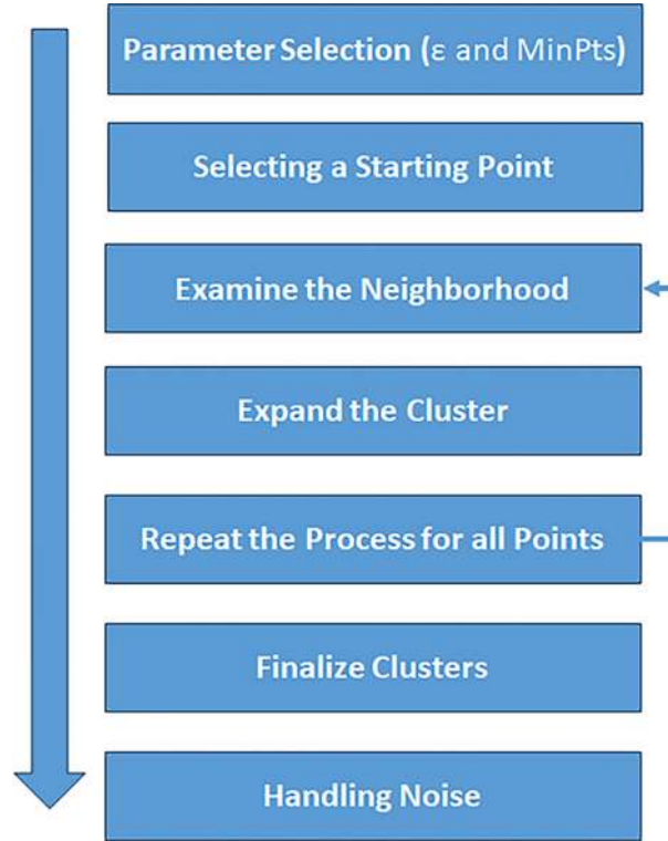
Figure 1. Logical flow chart of the DBSCAN algorithm.
