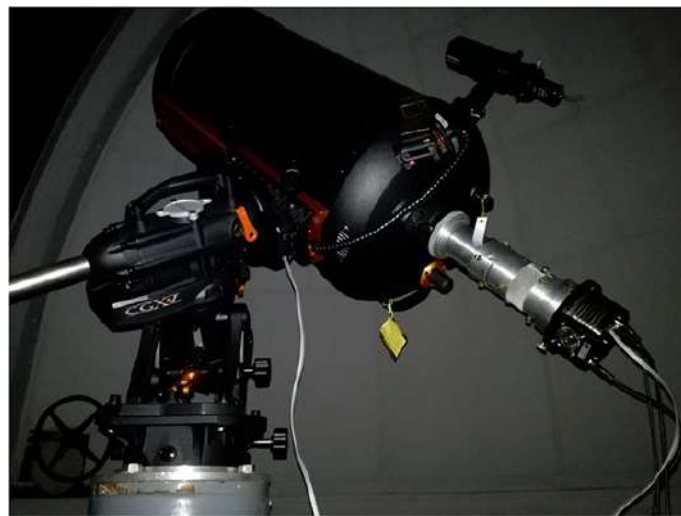
Figure 1. The Celestron SCT-14 telescope of Georgian National Astrophysical Observatory (Abastumani, Georgia) equipped with the PHISP and the Starlight Express SX-36 CCD
